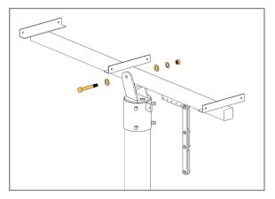
Secure Strongback to Mounting Sleeve with Pivot Bolt, two Flat Washers, Lock Washer and Nut. Secure Support Bar to Mounting Sleeve with 3/8" x 1-3/4" Bolt, two Flat Washers, Lock Washer and Nut.
