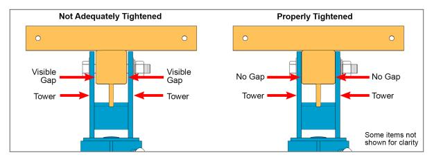
Tighten Pivot Bolt closing any visible gaps between the Strongback and the Mounting Sleeve Towers. **Torque to 125-150 ft.-lbs.**
