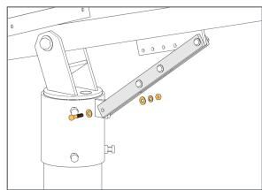
Torque Support Bar hardware at 32-34 ft.-lbs.
