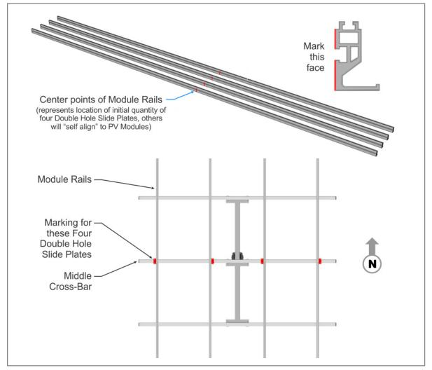
Locate the center of the Rails and mark as shown above. These marks are for the four (one-per Rail) Double Hole Slide Plates only. The additional Slide Plates do not require marks as they will be aligned to the Module mounting holes as the Modules are installed.
