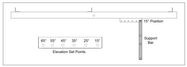
B. Tilt the rack to the desired elevation angle (15°, 25°, 35°, 45°, 55° or 65°) and reinstall the 3/8" hardware securing the Support Bar to the Strong-
