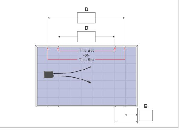
The dimensions must be taken from the site-specific Modules. The dimensions will be used to calculate the Module Rail positions.
