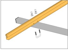
Hex Nuts at each Cross-Bar. Finger tighten for now to hold in place. Final tightening will come later.
