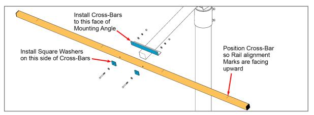
Install the three Cross-Bars with 3/8" x 3-1/4" Hex Bolt, Square Washer, Flat Washers, Lock Washer and Hex Nut. Tighten and **torque to 30-32 ft-lbs.**
