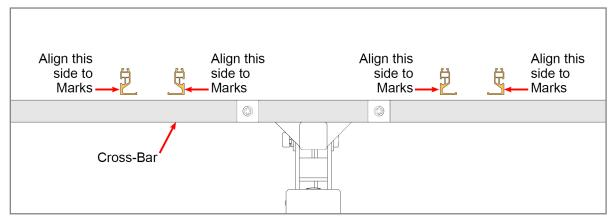
Be sure to align the correct side of the Rail with the Rail alignment marks on the Cross-Bars.
