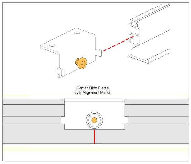
On each of the four Rails, install the two Double Hole Slide Plates to be centered over the previously made marks on the Rails. Insert the head of the Hex Bolt into the Rail channel as shown and align their centers over the marks. Tighten these eight Slide Plates securely and **torque at 32-34 ft.-lbs.**
