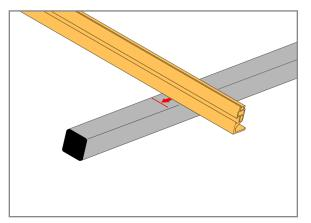
Align the Rail to the alignment marks and straddle its mounting holes over the Cross-Bar. Secure with 3/8" x 2" x 2-5/8" U-Bolt, Flat Washers, Lock Washers and
