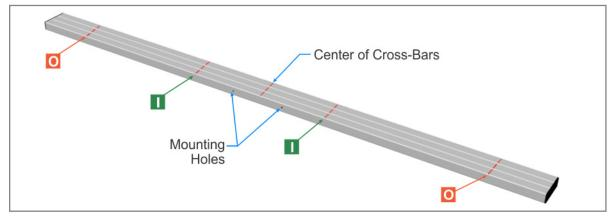
Measure and mark the center of the Cross-Bars then use the calculated dimensions I and O from the previous page to mark off their respective Rail positions. The image below shows these marks and their relationship to the Cross-Bars and Rails after assembly.
