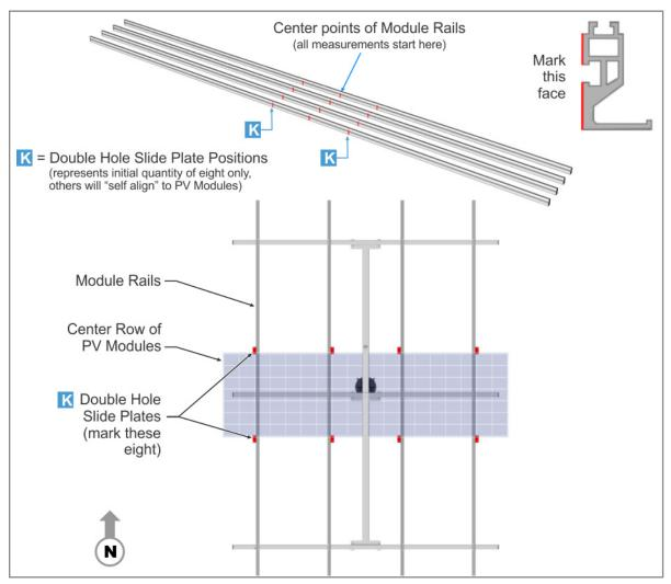
Locate the center of the Rails and mark as shown above. These marks correspond to the "K" dimension representing the locations for the eight Double Slide Plates (two-per Rail). The remaining Slide Plates do not require marks as they will be aligned to the Module mounting holes as the Modules are installed.
