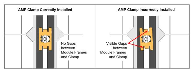
AMP Clamp bonding Mid Clamps must be installed as shown at above left and not as shown to the right. There cannot be any visible gaps between the bonding Mid Clamps and module frames.
