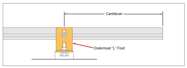
The POWER RAIL overhangs beyond the outermost "L" Foot. This overhang is referred to as "cantilever", or abbreviated as "C'ver". The distance between adjacent "L" Feet is referred to as "span". The length of both the cantilever and the span are dependent on
