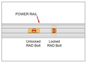
AMP Clamp bonding Mid Clamps are inserted into the POWER RAIL and positioned between adjacent Modules. Insert the 5/16" RAD Bolt into the POWER RAIL
