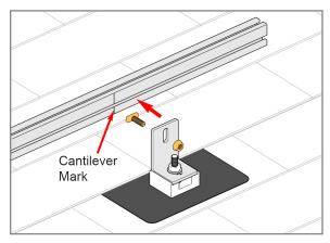
Foot with the cantilever mark on the POWER RAIL. Secure the POWER RAIL to the "L" Foot with the 5/16" Flange Nut. **Torque to 15 ft.-lbs.**
