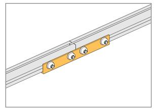
lock the Turn Bolts in place. Align the Splice Plate with the center of splice and secure to the POWER RAIL with the 5/16" Flange Nuts. **Torque to 15 ft.-lbs.**
