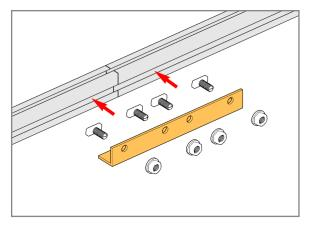
Splice Plates come in two configurations: 2-hole or 4-hole (above is a 4-hole). Insert a 5/16" x 3/4" Turn Bolts into the POWER RAIL and rotate 90-degrees to
