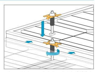
and rotate 90-degrees clockwise to lock the RAD Bolt within the POWER RAIL. Push the Modules against the AMP Clamp. Tighten the 5/16" Flange Nut. **Torque to 15 ft.-lbs.**
