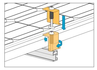
RAD End Clamps are used on the outer Modules. Insert the 5/16" RAD Bolt into the POWER RAIL and rotate 90-degrees clockwise to lock the RAD Bolt within the POWER RAIL. Secure with the 5/16" Flange Nut. **Torque to 15 ft.-lbs.**
