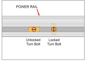
Insert the 5/16" x 3/4" Turn Bolt into the POWER RAIL and rotate 90-degrees, locking the Turn Bolt in place. On the outermost "L" Feet, align the center of the "L"
