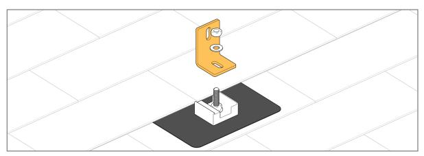
Secure "L" foot to appropriate anchoring device per the manufacturers instructions. Above is shown using the POWER RAIL PV Flash and attaching hardware.
