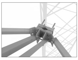
Step #7 To adjust the Antenna Mount from 10' to 12', or 15' configurations loosen the four 5/8-11 x 5-1/4" bolts and telescope both outer square tubes outward.
