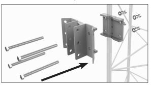
Step #4 After the main structure tube is inserted, install the two 5/8-11 x 5-1/4" bolts and torque to 60 ft-lbs.
