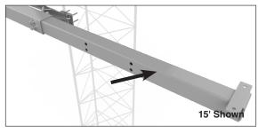
Reinstall and torque the two 5/8-5–1/4" bolts to 60 ft-lbs.
