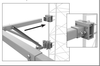
**Step #5** If the tower support structure interferes with the lower tower mount, it can be adjusted up 3" or down 3".
