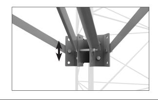
Step #6 Next, align the angle support structure with the appropriate holes. Install one 5/8-11 x 5-1/4" bolt, flat washer, lock washer and nut through the two center angle support brackets and the center of the lower tower mount. Then install the outer two 5/8-11 x 1-1/2" bolts, flat washers, lock washers and nuts. Torque all three 5/8" - 11 bolts to 60 ft-lbs.
