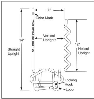
The Hook/Loop feature is located on the front and back of the BPD Crossarm.
