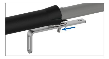
Trim the other set of strength members flush with the end of the strength member bracket. Once the strength members are trimmed, remove the strength member bracket from the cable.
