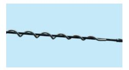
ADSS cables tend to vibrate at higher levels due to their light weight, compared to other cables of the same size. The FIBERLIGN® Spiral Vibration Damper reduces levels of Aeolian vibration on ADSS cables without the need to calculate precise positioning.
