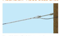
The FIBERLIGN® Dielectric Dead-end has been designed to terminate ADSS aerial fibre optic cable securely and gently. The two-component design consists of structural reinforcing rods and a dead-end component to transfer tensile loads and distribute radial compressive forces without damaging the fragile, internal optical fibres.
