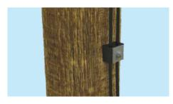
The FIBERLIGN® Downlead Cushion secures both the ADSS cable downleads to the structure, while minimising the compression force from the clamp that could be transferred to the optical elements.
