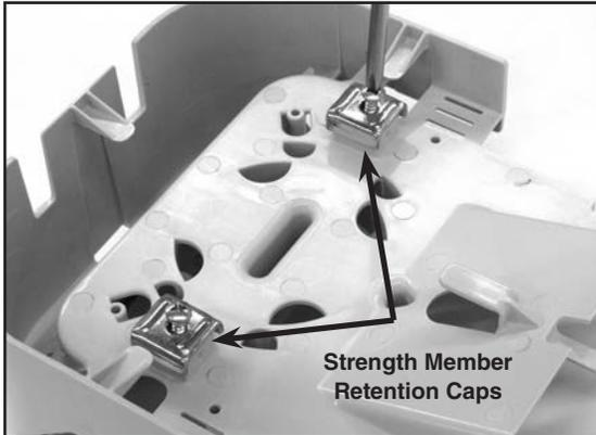
**Step #9** If the cable contains Kevlar®, wrap the braided Kevlar around the screw under the retention cap. Position the cable strength members under the cap and tighten down the screw to secure them.
