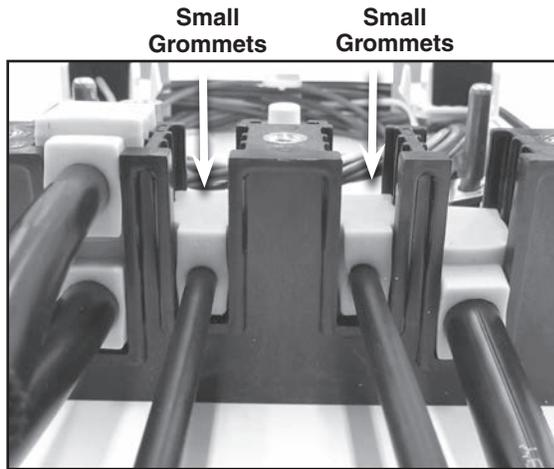
**IMPORTANT NOTE:** When installing the small grommets, position them in the pockets as shown below.
