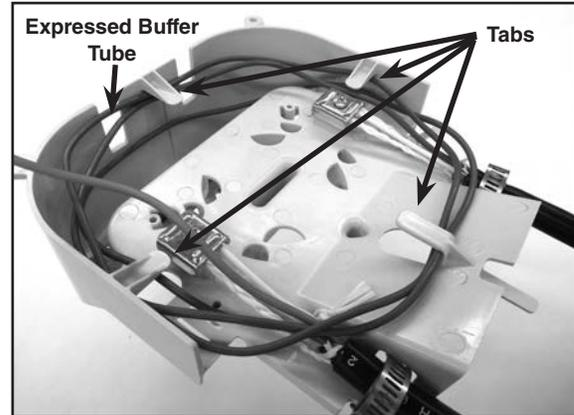
**Step #12** Route any buffer tubes with fibers to be spliced under the tabs once before routing them to the top of the organizer.
