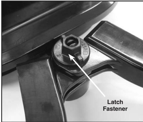
**Step #55** Secure the collar latch and insert the pin into the latch.
