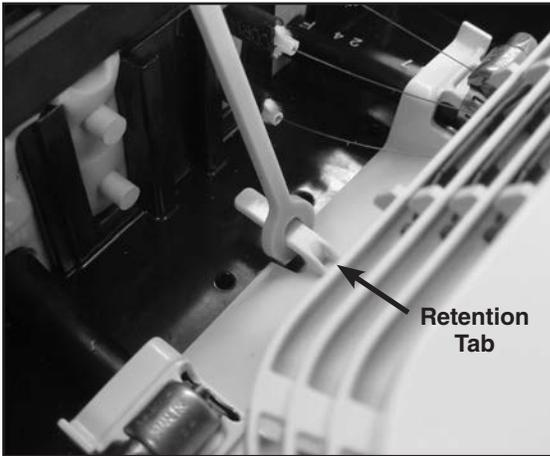
**Step #49** Secure the splice trays by placing the loop of the tether over the button heads of the organizer as shown below.
