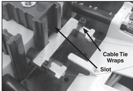
**Step #39** Install the four position cable restraint bracket in the slot of the base as shown below. Use a cable tie wrap(s) to secure the drop cable(s) to the restraint bracket.
