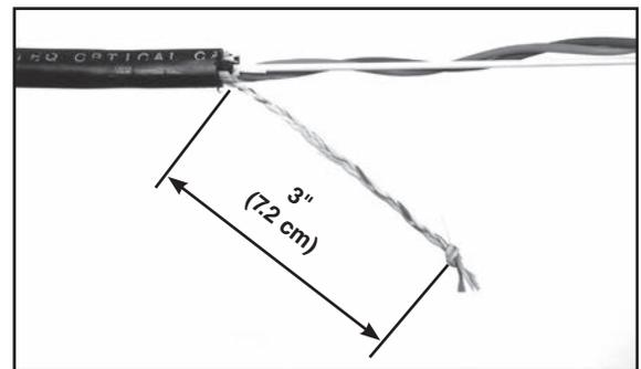
**Step #7** Trim the cable strength member 2.5" (6.4 cm) away from the cable sheath opening.
