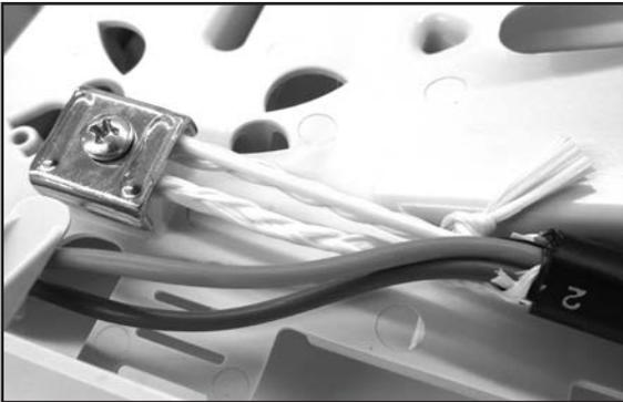
**Step #10** Secure the cables to the organizer with hose clamps as shown below.
