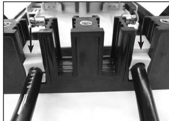
**Step #25** Secure the organizer to the base with the self-tapping screws that are provided.
