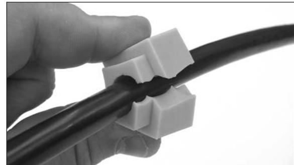
**Step #3** If the cable has a tracer wire or is a Figure 8 style cable, remove the ground wire or tracer wire from the portion of the cable that will be positioned in the grommet and insert the cable into the grommet.
