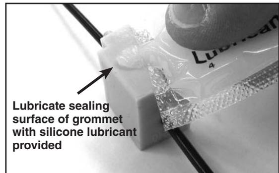
**Step #36** Install the bottom layer of small grommets in the inside grommet pockets of the closure as shown below.
