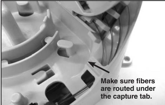
**Step #21** Route dark fibers from the feed buffer tube(s) in the dark fiber storage area of the organizer.
