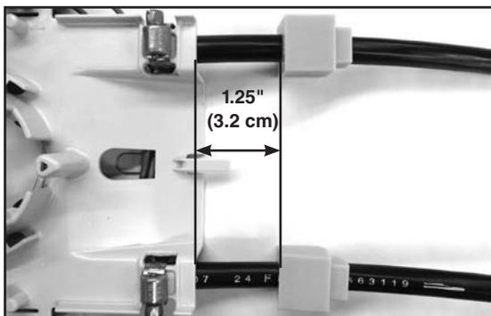
**Step #23** Apply a light coating of lubricant to all outer surfaces of each grommet.
