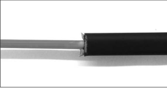
**Step #31** Mark and remove the buffer tube 1/8" (.32 cm) away from the sheath opening.
