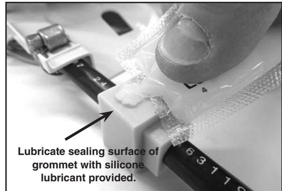
**Step #24** Insert the grommets in the outside grommet pockets of the closure as shown below.
