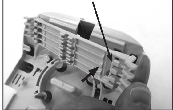
**Step #18** Place the first splice tray at the bottom of the hinge plate and position the splice tray perpendicular to the organizer as shown below. Make sure that the back side of the splice tray is facing up.
