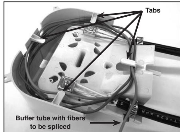
**Step #13** Wrap the buffer tube(s) with felt and secure the buffer tube(s) to the organizer with 2 tie wraps.
