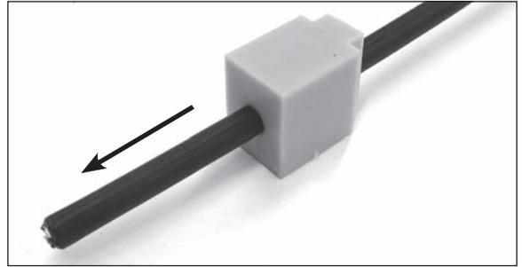
**Step #28** If the cable has a tracer wire or is a figure 8 style cable, remove the tracer wire or messenger wire from the portion of the cable that will be positioned in the grommet and insert the cable into the grommet.
