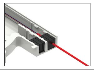
**Step #5** If a splitter tray is being used, insert the splitter(s) into the splitter block(s).
