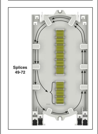
**Step #8b** Outgoing Fiber Routing for Long Splice Trays
