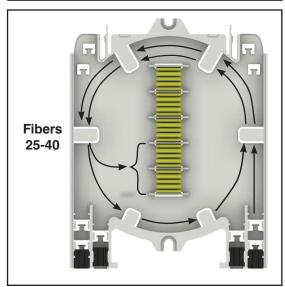
**Step #6b** Outgoing Fiber Routing for Short Splice Trays
