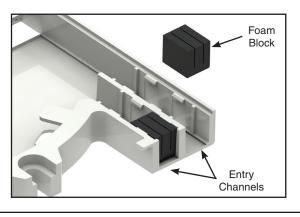
Step #3 Insert the LITE-GRIP splice blocks between the guide ribs and confirm that the edges of each LITE-GRIP splice block are captured within the slots of the guide ribs.
