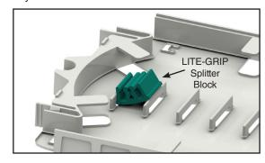
Step #4 Insert the microtube(s) or tight buffer tube(s) into the slot(s) of the foam block(s).
