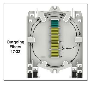
**Step #8a** Incoming Fiber Routing for Long Splice Trays
