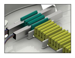
**Step #6a** Incoming Fiber Routing for Short Splice Trays
