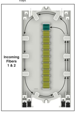
**Step #9b** Outgoing Fiber Routing for Long Splitter Trays
