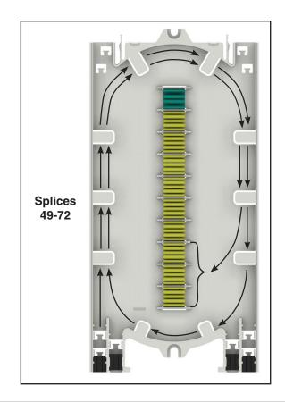
Step #10 Install the cover onto the tray by first capturing the legs of the cover under the tabs of the tray. Once the legs are captured, rotate the cover downward until the locking tabs of the cover snap into place in the tray.
