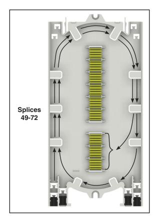
**Step #9a** Incoming Fiber Routing for Long Splitter Trays
