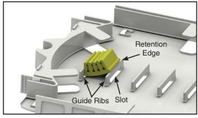
**NOTE:** If a splitter tray is being used, install the LITE-GRIP splitter block(s) in the top slot(s) of the tray as shown below.
