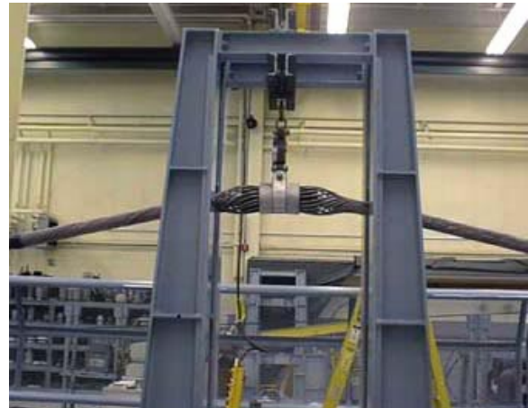
Laboratory Testing of THERMOLIGN Suspension
