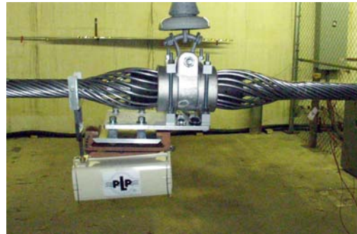
Figure 21 – Ontario Hydro Vibration Recorder Mounted on ARMOR-GRIP Suspension
