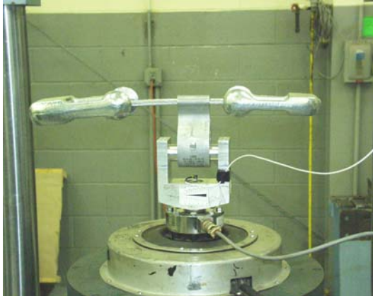
Figure 16 – Damper Response Test Set-Up
