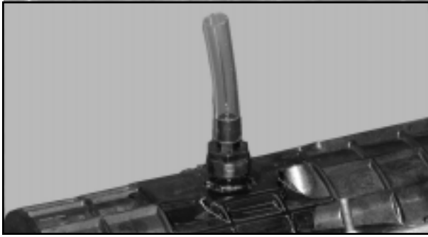
FIGURE 3 - PRESSURE RELIEF VALVE ON ARMADILLO CLOSURE
