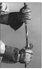
**Step #8** Position the center of the second element at the joined ends of the wire rope.
