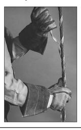
**Step #11** Position the center of the third element at the joined ends of the wire rope.
