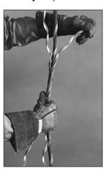
Step #13 Grasping the second and third elements, simultaneously wrap them onto the bottom rope.
