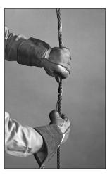
Step #6 Wrap the lower portion of the first element onto the bottom wire rope, pulling slightly away from the rope while applying.
