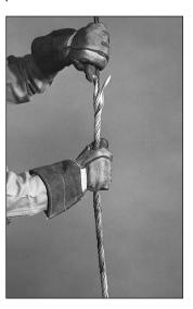
**Step #17** A complete marriage of elevator wire ropes shown below.
