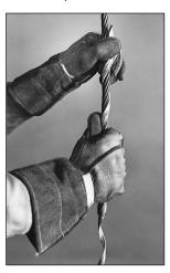
Step #5 Position the end of the bottom wire rope approximately 1/16 of an inch from the end of the upper wire rope.
