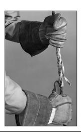
**Step #15** Grasping the second and third elements, simultaneously wrap them onto the top rope.
