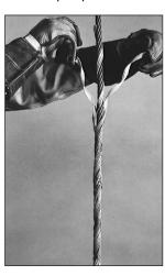
Step #16 Snap on the two ends with thumb pressure.
