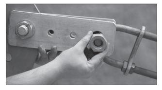
Step #4 Tighten nut and bolt and fully insert the cotter pin. Ensure that plates are parallel to each other and that the head of the bolt is tight against washer and plate.
