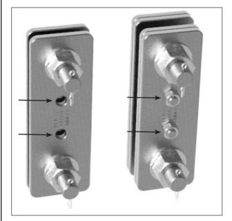
Step #2 Line up one of the larger holes with the anchoring hardware and insert the bolt through both link plate then install the nut. Be sure that the plate markings are facing outward.
