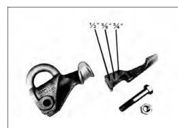
1. Component Parts: The keeper is to be used with 1/2", 5/8", and 3/4" anchor rods (see arrows). For 1" and 1-1/4" anchor rods, the PREFORMED Pulling Eye is used without the keeper.
