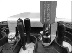
Step #2 Mount the Dome Bracket to the closure by using the raised bolt mount molded into the dome. Secure the bracket using the provided self-tapping bolts, making sure to keep the bracket spaced evenly between the bolts.
