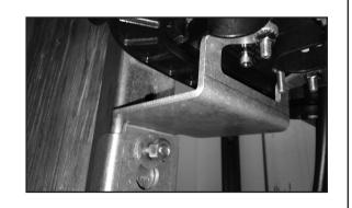
Step #6 Position the Dome Bracket in place and tighten the upper bolt. Once secure, return to the lower bolt and fully tighten.
