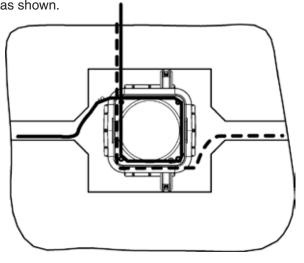
**Step #14** Drive stakes until the base is captured by the anchor plates of the stakes and remove driver cap from stakes.
