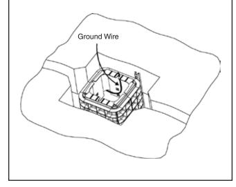
**Step #13** Make sure the cable is entering the base in opposing corners and route cable in base as shown.
