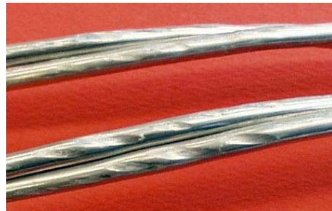
Figure 9 – Notching of Aluminum Strands Under Bolted Suspension Clamp
